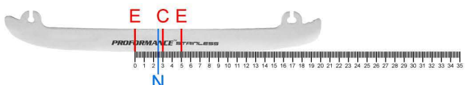
A flat forward lean glide surface of 50 mm shifted 5 mm towards the front (end points are located 30+20 mm from center point). The new center (N) should be centered between those end points (moved 5 mm towards the front).
