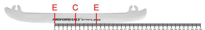
A radius glide surface with end points that are located 50+50 mm from center point. Note, if you want to pitch it, grinding will occur outside one of the markings.
